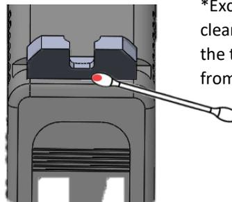
\*Excessive cleaning can pull the threadlocker from joint
