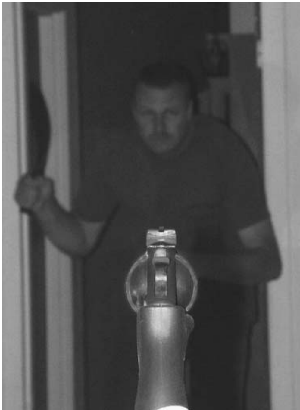
Here, a conventional blade front and square notch rear sight is seen on the same target. For clarity this photo was taken with a lot of light on the handgun. Under most circumstances, the sights may not have this much contrast.
